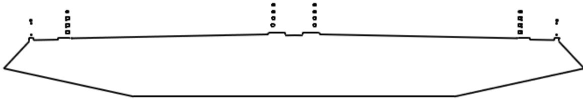
Figure 1. Schematic diagram of the main girder.
